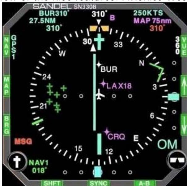
**The Sandel can be installed over a dozen different ways.** It can be a stand-alone HSI that works with a fluxgate, a Bootstrap off
