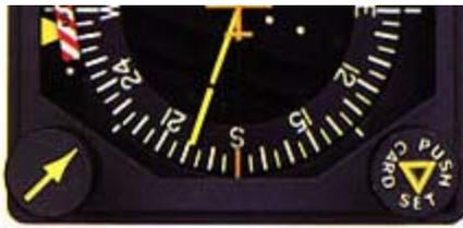
again. This HSI, slaved or not, **MUST** have BOTH vacuum and electrical inputs in order to operate. In other words, if you lose vacuum or the electrical system, this HSI compass card will quit! Expect to pay between \$300-500/year to keep your NSD repaired. Sure, you may not need a repair for several years but when your unit does, it really hits the ole pocket book. A new, slaved NSD-360 sells in the neighborhood of \$6,900.00 plus installation.
