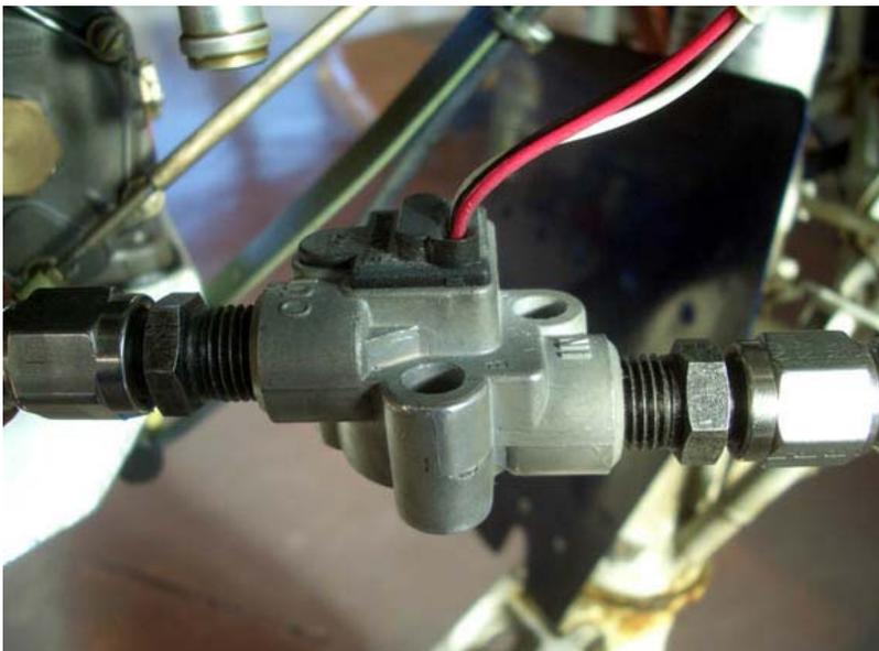
which was designed for the boat business and is resold with “aviation paperwork” and at the customary inflated price by the flow indicator manufacturers. The 201B generates around 30,000 pulses per USG/hour; the actual figure (called the “K-factor”) is supposed to be individually measured and marked on each unit. This K-factor is configured in the instrument, and the result should be an accurate fuel flow indicator system.
