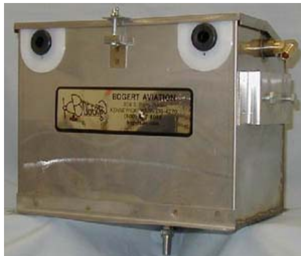
Repairing a battery box is a minor repair. If beyond repair, consider a PMA replacement (shown here) or a serviceable part from a salvage yard.
