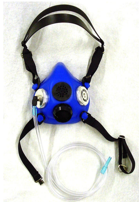
Figure 3. MH oro-nasal mask. The oxygen delivery pressure sensing line connects to the mask at the right cheek fitting. Mask features a voice transmitter (located at the nose of the mask) to propagate voice transmission through the mask and support use of a standard aircraft communication headset with boom-type microphone. A flapper-type exhalation valve is located at the lower center part of the mask, and an inhalation valve with flapper is located on the left cheek of the mask.
