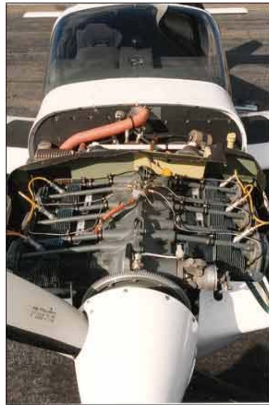
Power is provided by the Lycoming IO-540 series, a reliable if not economical choice.
