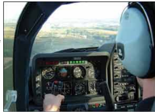
Cockpit visibility is good, but forward windshield post and door frame obstruct.
