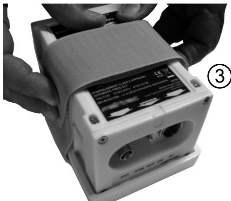
Figure 7: Installing the transmitter on the bracket
