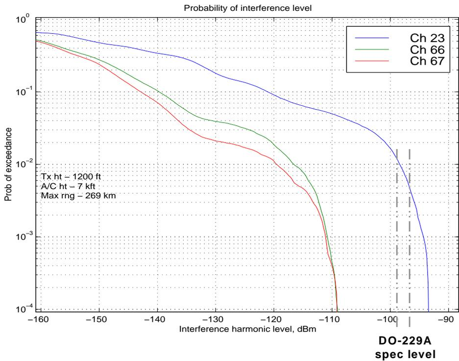
Figure 5-2 Probability of Receiving Interference Power at the Indicated Level
