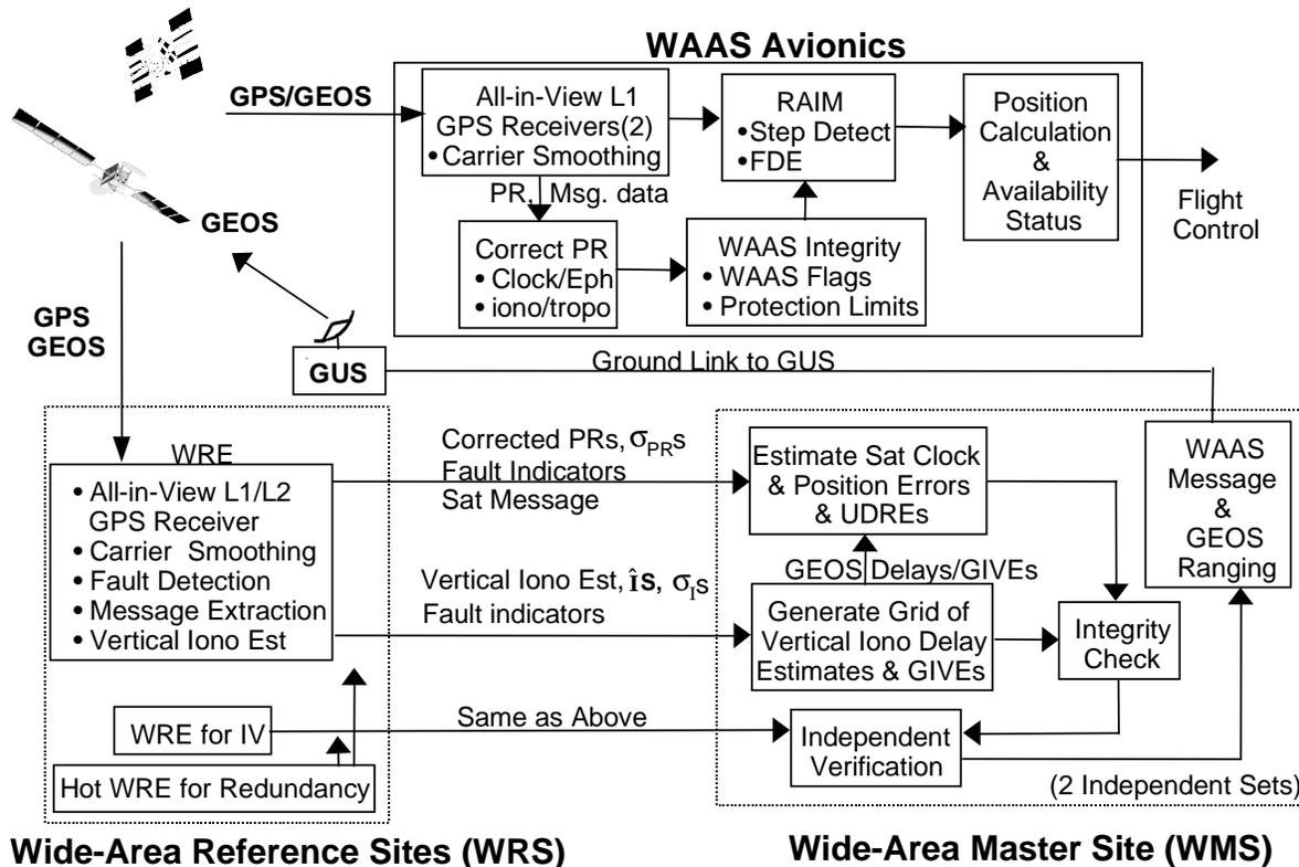
Figure D-1 GPS/WAAS Architecture
