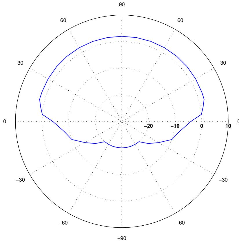
**Figure I-1 GPS Receive Antenna Gain (dBi) Elevation Pattern Used for All Interference Simulations**
