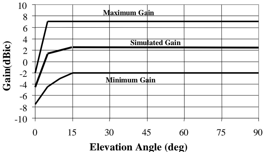
Figure C-2 Simulated Aircraft Antenna Gain
