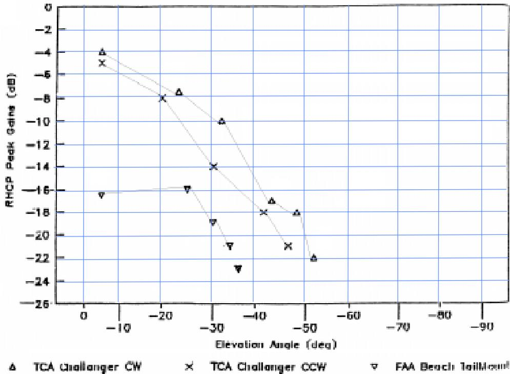
**Figure C-3 Measured Antenna Pattern Data**
