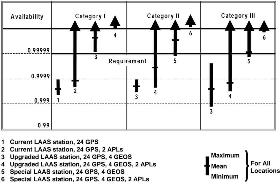
Figure 4-7 Analysis Results for Several GPS/LAAS Configurations
