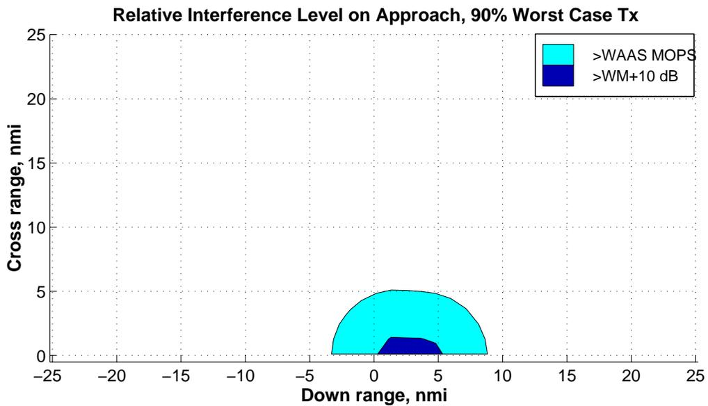
**Figure I-7 Simulation Results for Television Interference**
