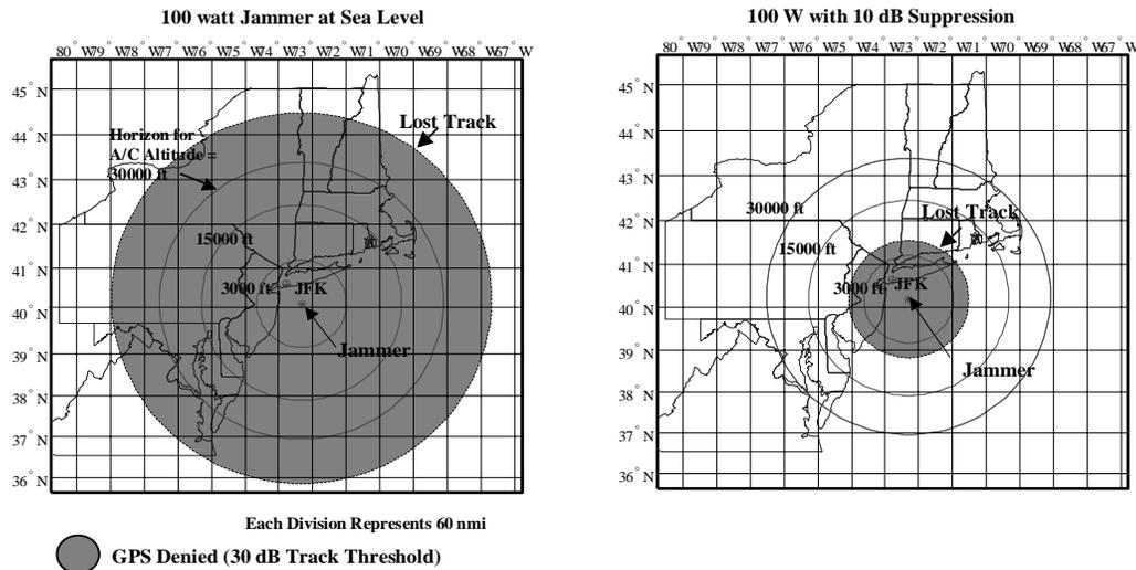
**Figure 5-4 Outage Area Caused by 100-W Jammer**
