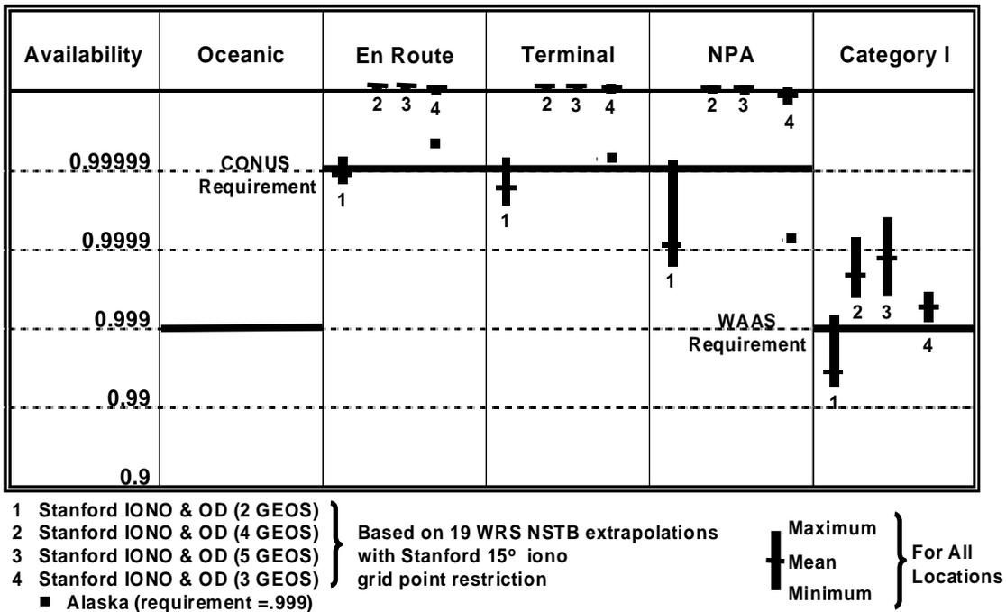
Figure 4-6 GPS/WAAS Results Versus GEOS Configuration Options
