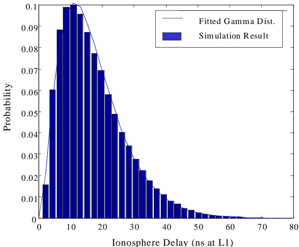
**Figure C-3 Gamma Distribution Fit to Simulated Monthly TEC Variation**
