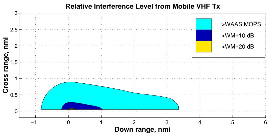
**Figure I-3 Simulation Results for VHF Interference**
