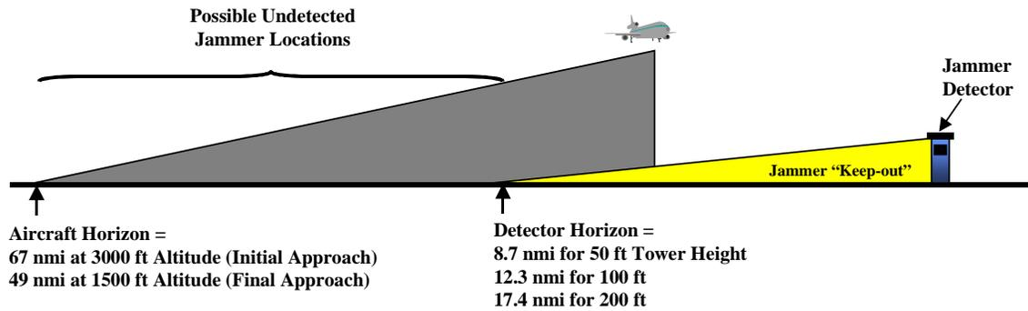
**Figure J-2 Detector Line-of-Sight Limit**
