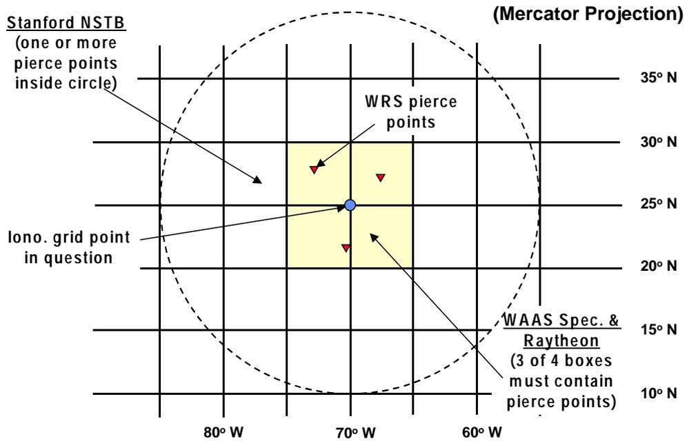
Figure D-3 Comparison of Proposed Ionospheric Gridpoint Validity Constraints
