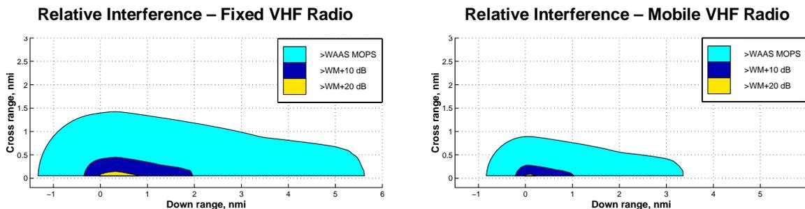
**Figure 5-1 Interference Zones for VHF Radio Transmitters**
