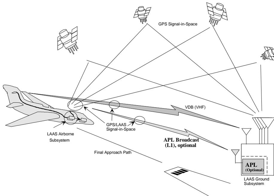
**Figure E-1 GPS/LAAS Relative Positioning Concept (from GPS/LAAS MASPS-7, 7/22/98)**
