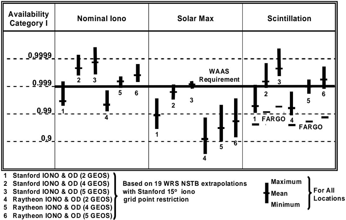
Figure 4-5 GPS/WAAS Results Versus Ionospheric and Orbit Determination Algorithms
