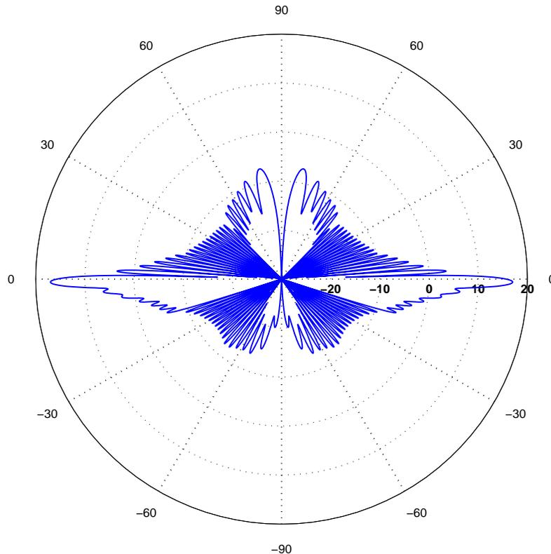
**Figure I-5 Television Antenna Gain (dBi) Elevation Pattern Used for Simulations**
