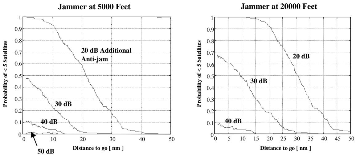
**Figure 5-9 GPS Outage Caused by 100-W Airborne Emitter**
