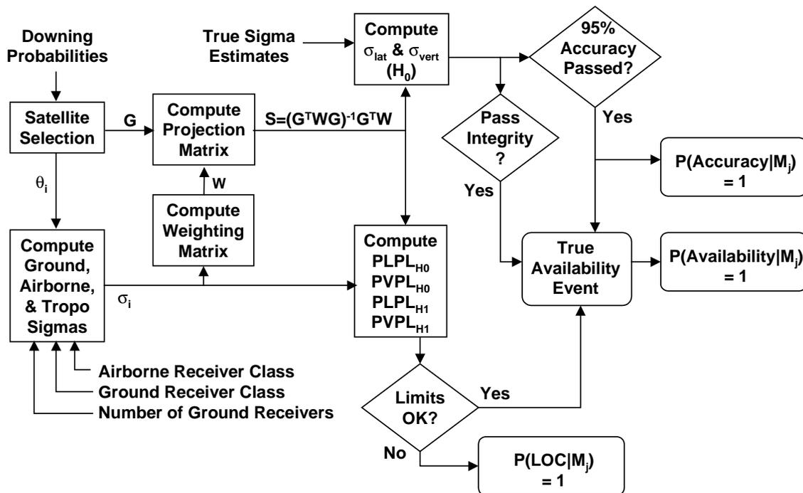
Figure E-3 GPS/LAAS Simulation Structure
