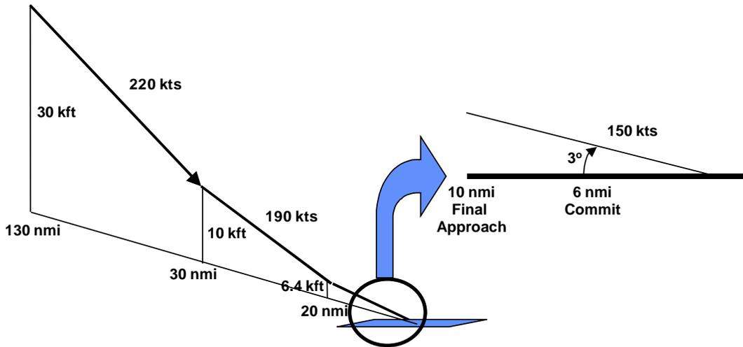
**Figure I-2 Approach Scenario Used for Interference Simulations**
