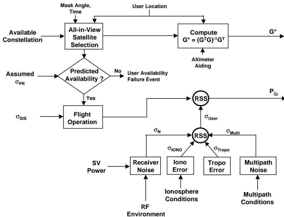
**Figure C-1 GPS Measurement Error Simulation Structure**
