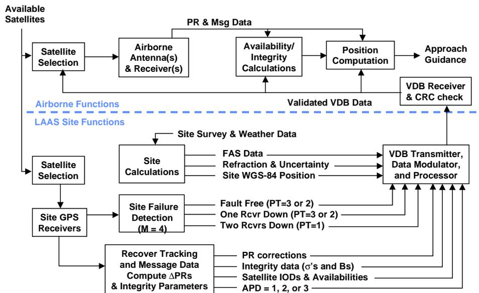
**Figure E-2 GPS/LAAS Functional Block Diagram**
