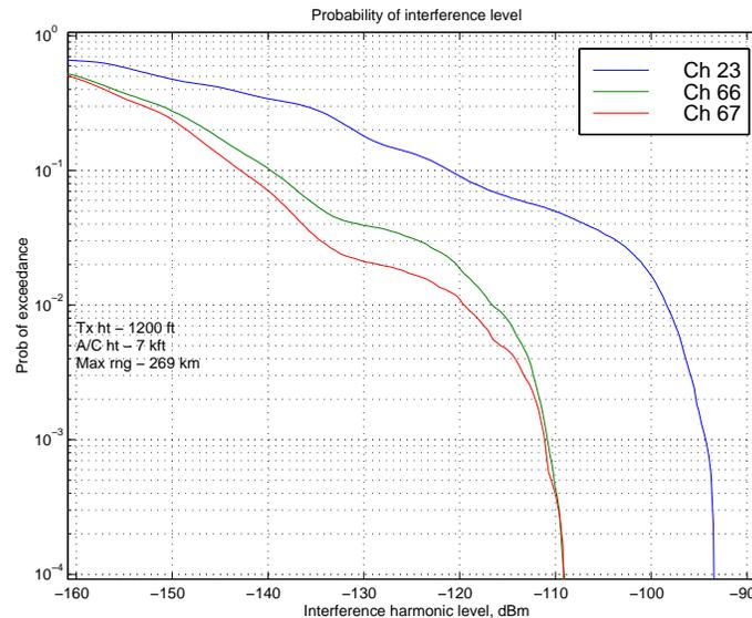
**Figure I-6 Probability of Received Interference Level, En Route GA Aircraft**
