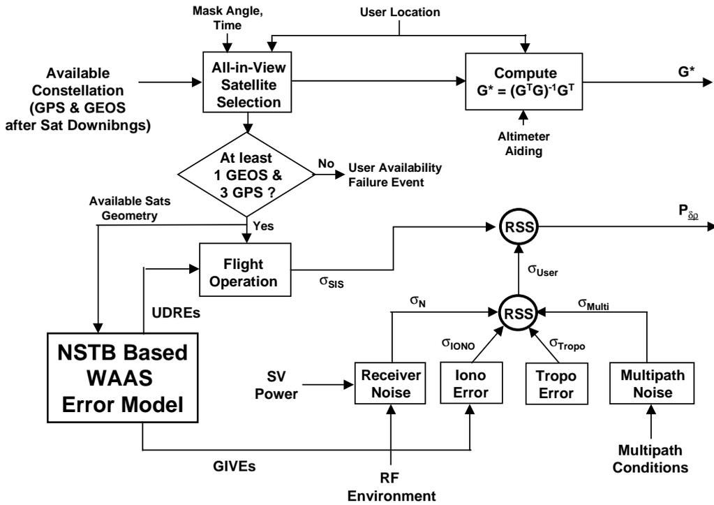
Figure D-2 WAAS Measurement Error Simulation Structure
