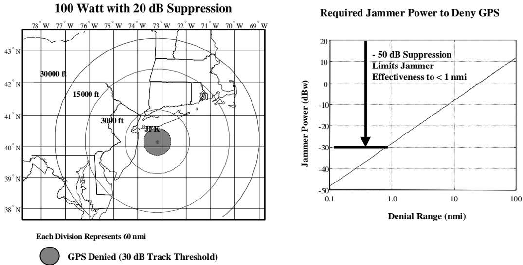
**Figure 5-5 A 100-W Jammer with Additional Interference Suppression**
