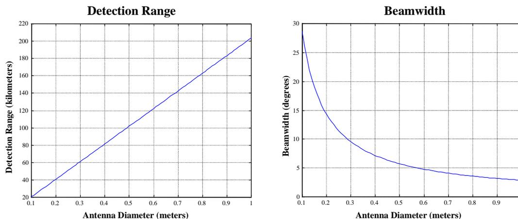
**Figure J-1 Detector Sensitivity and Beamwidth for a 1-Watt Emitter**
