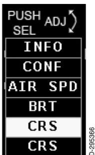
The left knob can be used to set the course pointer (**CRS**), set display brightness (**BRT**), set the airspeed bug (**AIR SPD**), Aircraft Configuration (**CONF**), and display the information screen (**INFO**). Detailed operation of each selection is provided later in this manual.
