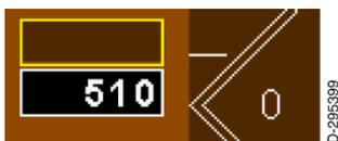
When a minimum altitude is set and the barometric altitude is within 50 feet of the set minimum, a yellow boxed window is displayed in the lower right corner of the ADI, above the Minimum Altitude Alert window, indicating the minimum altitude detection condition is armed.
