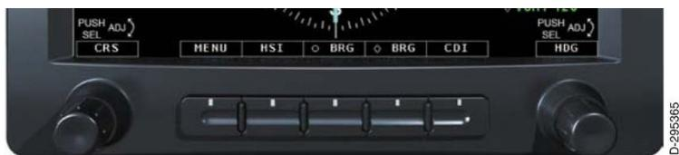
Figure 2-5 Rotary Control Knobs
