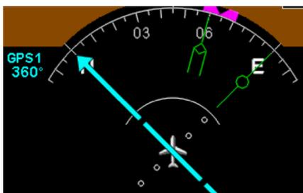
The selected course display consists of a digital readout and a cyan pointer. The pointer rotates within the compass rose. The selected course value is indicated at the top left of the HSI.
