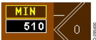
When the barometric altitude is equal to or less than the approached minimums set value, "MIN" is displayed in the annunciator box.
