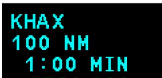
The waypoint identifier and distance readout are displayed near the upper right corner of the HSI. The source for this data is GPS only. The KFD 840 does not display any DME data.
