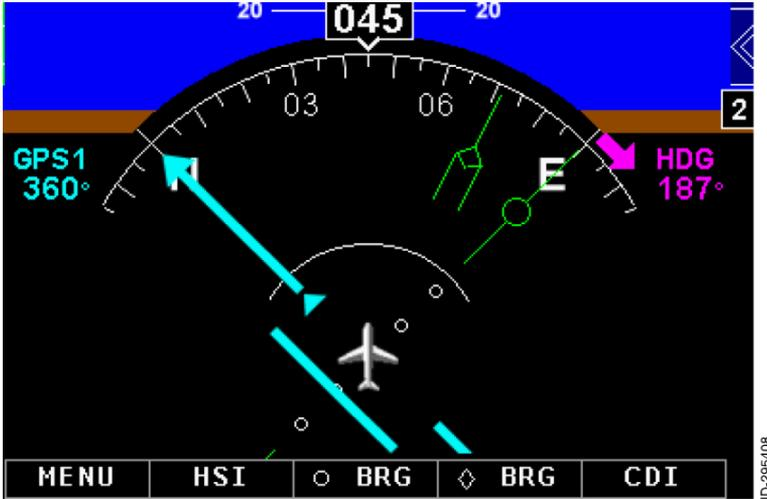
Figure 7-4 Heading Select Bug Off-Scale
