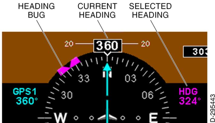
**Figure 7-3 Selected Heading Readout and Bug**
