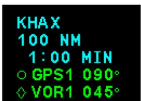
The bearing pointer source is selected with the **O BRG** and **◊ BRG** soft keys on the unit. The digital bearing to the station is displayed next to the selected source. If the bearing data is invalid the readout displays amber dashes.
