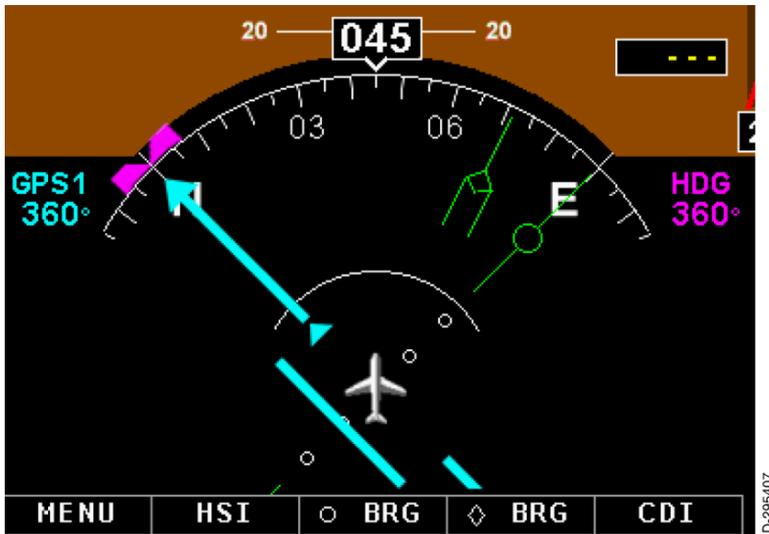
**Figure 7-2 Partial Compass (ARC HSI)**
