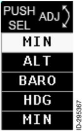
The right knob can be used to control the heading bug selection (**HDG**), set the baro settings input (**BARO**), set the selected altitude bug (**ALT**) and set the minimum altitude alert (**MIN**). Detailed operation of each selection is provided later in this manual.
