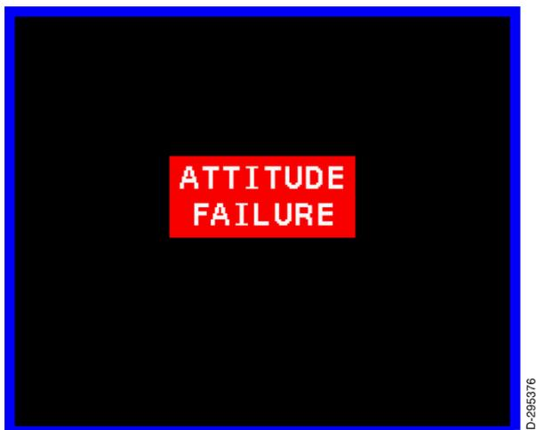
**Figure 3-4 Attitude Failure Indication**
