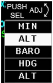
Press the right knob three times to activate the Altitude bug **ALT**. Turn the knob clockwise to increase the **ALT** bug setting and counterclockwise to decrease the value.
