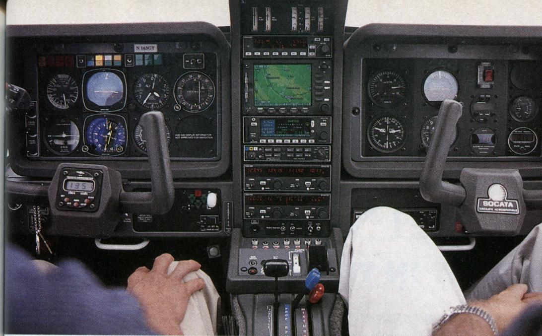
The standard avionics package in the Trinidad GT includes the new Bendix/King KMD 150 multifunction display. The KFC 225 automatic flight control panel is mounted at the top of the radio stack where it is easy to see.
